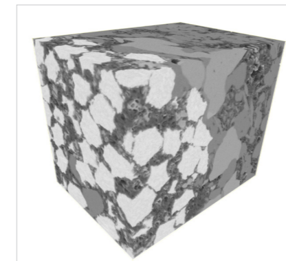
ZEISS Crossbeam 550 FIB-SEM – 2.5 nm voxel size
