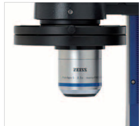
Objective PlanApo S 3.5x mono on Objective slider S/doc ■ For axial mode only ■ Free working distance FWD= 16 mm ■ Max. possible resolution of 1,510 LP/mm (equals 0.3 μm)
