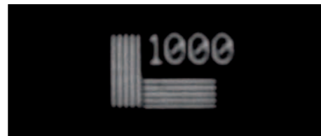
Combine SteREO DiscoveryV12 with the PlanApo S 2.3x objective to obtain resolutions of up to 1,000 line pairs per millimeter (LP/mm).
