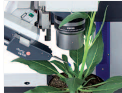
The large space between the objective and the stage can be used to handle all types of specimens. You can even isolate trichomes from tobacco plants if need be!
