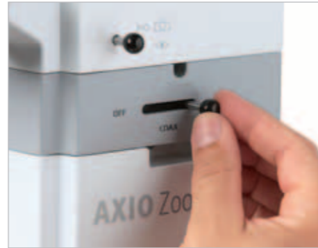
Use the slider to turn off the coaxial epi-illumination. Use this free position for other illumination methods.
