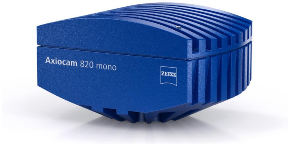
Axiocam 820 mono 20 megapixel camera is equipped with a large 17.5 mm diagonal back-illuminated CMOS sensor having a peak quantum efficiency of 86 %. In combination with its low readout noise, this camera is the perfect choice for imaging faint fluorescence signals in living or fixed samples. Its square sensor most efficiently utilizes the optical field of view of the microscope for capturing more details.
