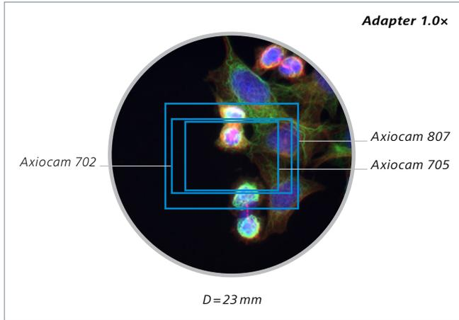
Typical image sensor diameters are 7.9 mm (1/2" format), 11 mm (2/3" format) or 16 mm (1" format).
