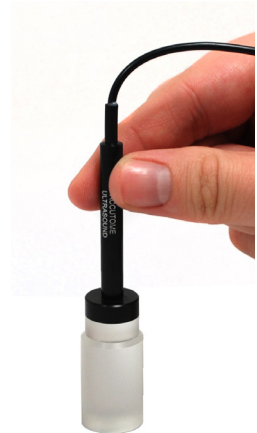
Figure 9.6 - Using the A-Scan Test Block
