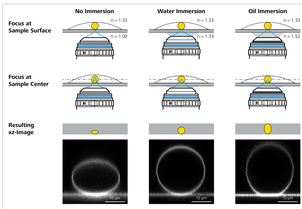
XZ projection of a giant unilamellar vesicle prepared from the lipid DOPC doped with an Atto647N-labeled lipid, imaged with a 40x/0.95 air objective (left), a 40x/1.2 water immersion objective (middle) and a 40x/1.4 oil immersion objective (right).
